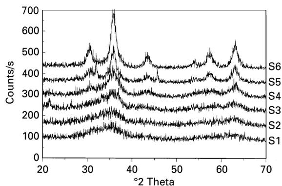
Fig. 1. X-ray powder diffraction patterns for the as-precipitated nanoparticles shown in Table 1 under different pH and NaOH concentration conditions.
