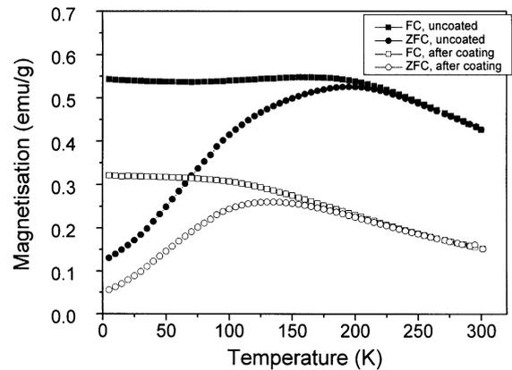
Fig. 3. Magnetization vs. temperature measured at 10 Oe in the zero-field-cooled and field-cooled states for nanoparticles (S6) before and after being coated with sodium oleate.
