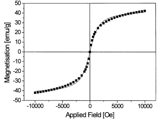
Fig. 5. Magnetization vs. applied magnetic field for nanoparticles (S6) without coating at  $300 \text{ K}$ . Experimental (solid rectangle) and calculated (solid line) data represent the best fit for the Langevin function.
