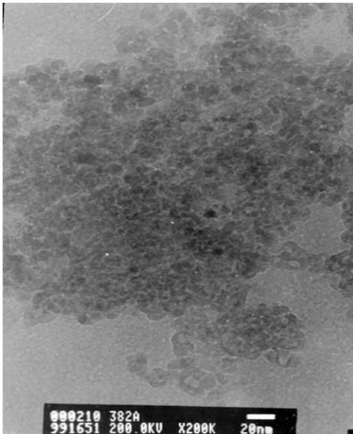
Fig. 2. TEM micrograph of  $\text{Fe}_3\text{O}_4$  nanoparticles (sample S6, Table 1).
