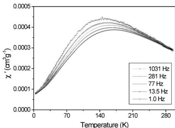
Fig. 6. AC-magnetic susceptibility data for nanoparticles (S6) coated with sodium oleate measured in the frequency range 1–1031 Hz.
