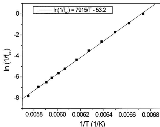
Fig. 7. Temperature dependence of the relaxation time of the magnetization estimated from AC-magnetic susceptometry data for nanoparticles (S6) coated with sodium oleate measured in the frequency range 1–1031 Hz.
