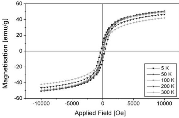
Fig. 4. Magnetization vs. applied magnetic field for nanoparticles without coating (S6).
